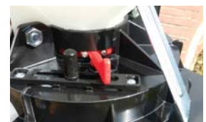
Flow Limiter Stop Set the hopper opening to a fixed position for consistent delivery of material to the propeller
